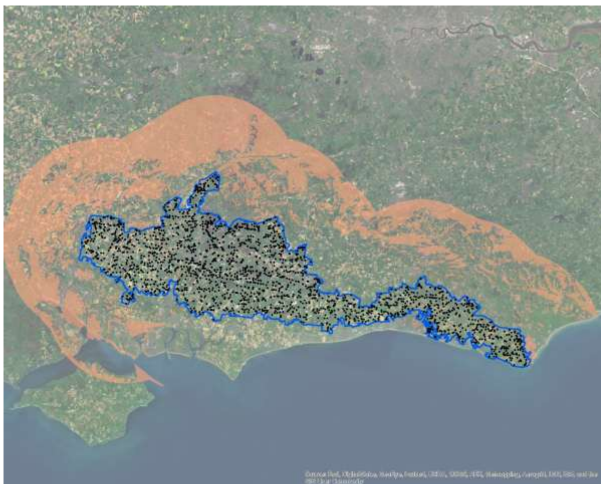
Figure 1 Viewshed based on 2,263 points on the 5m DTM (Red is not Visible).
